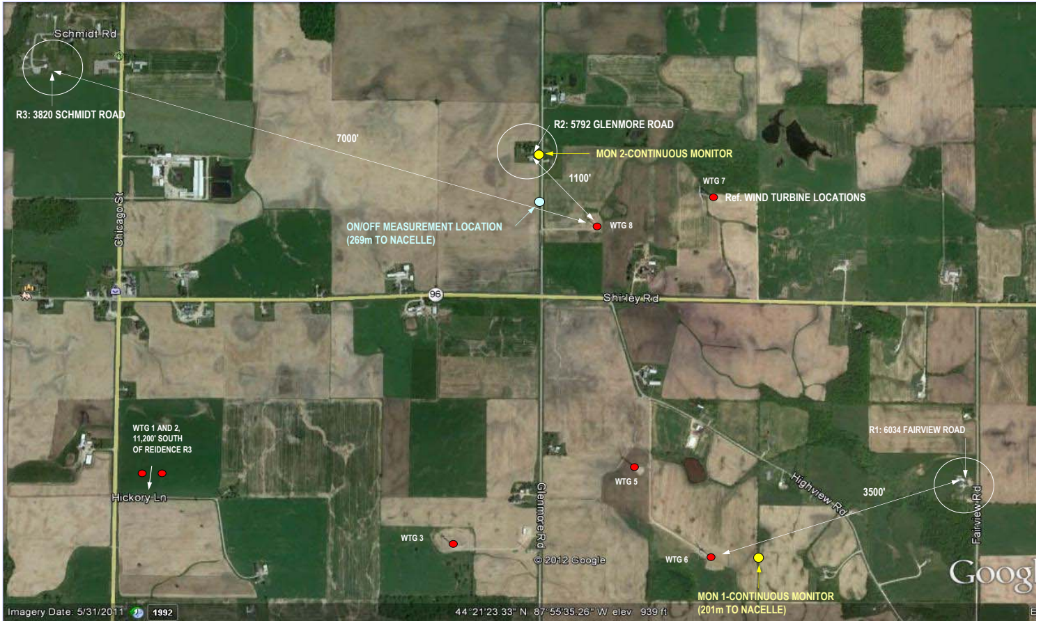
Figure 2.1: Aerial view showing sound survey locations
